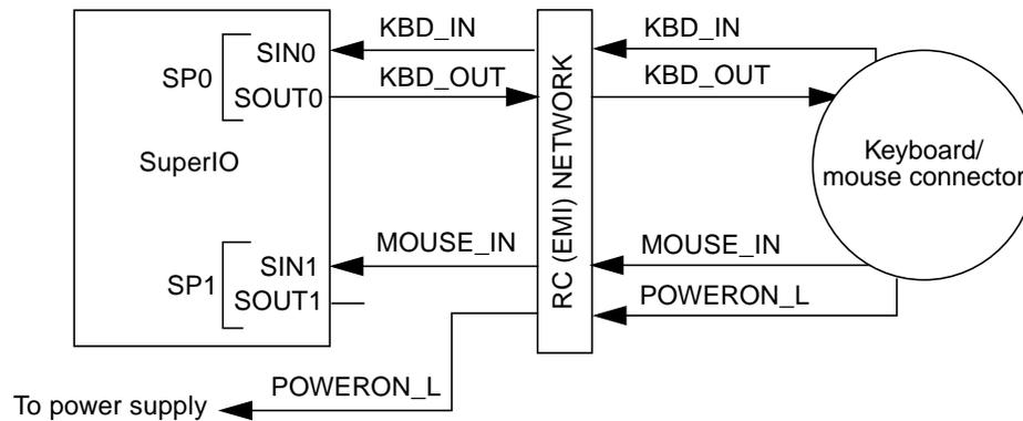
FIGURE C-11 Standard Serial Port Functional Block Diagram
