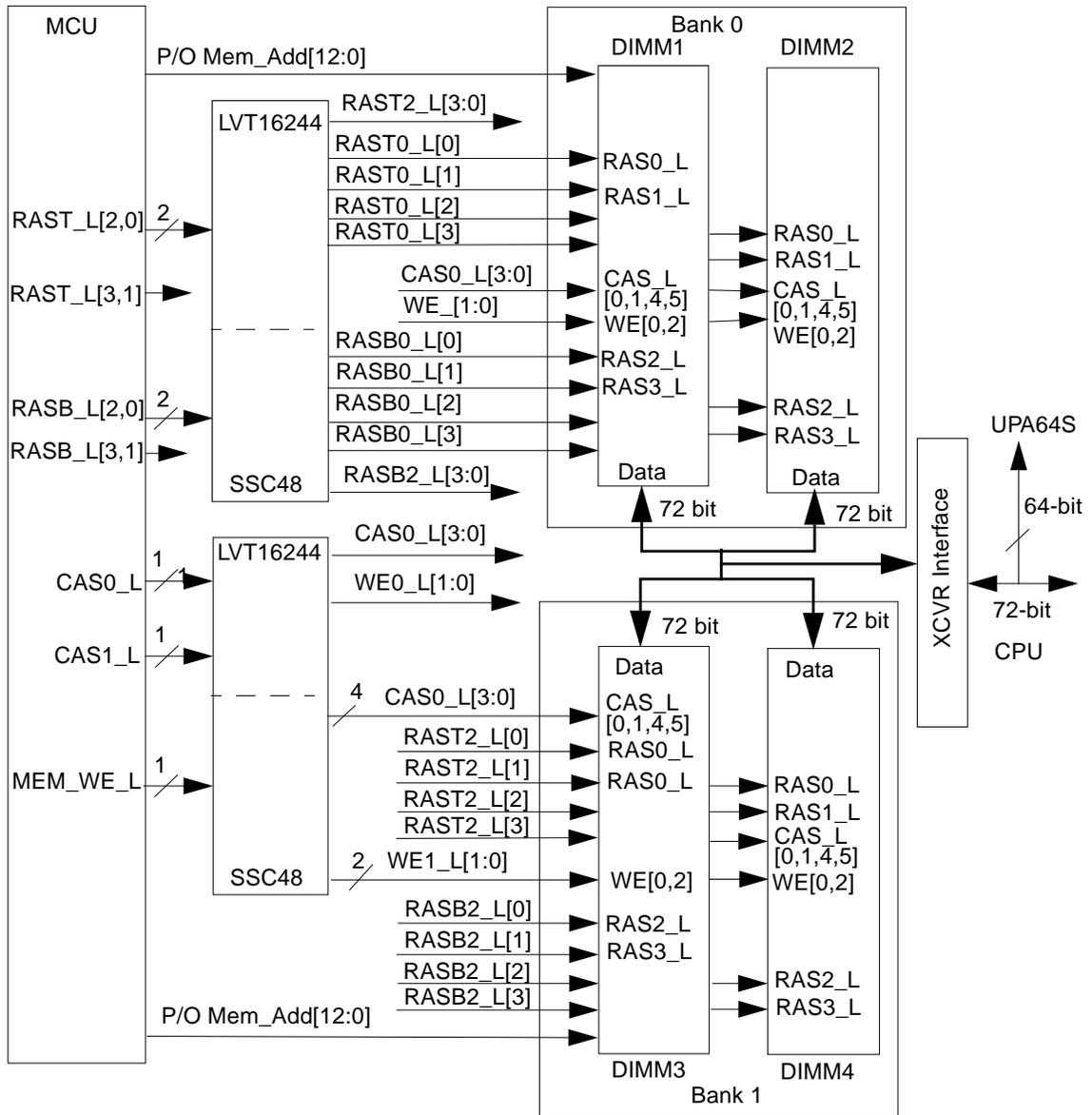
FIGURE C-9 Memory Interface Functional Block Diagram
