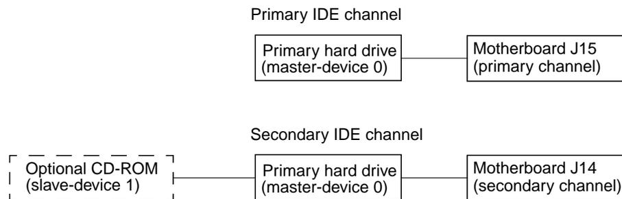
FIGURE 7-7 Hard Drive Mirroring Configuration
