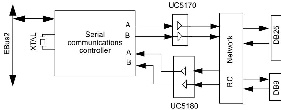
FIGURE C-12 Communications Controller Serial Ports Functional Block Diagram
