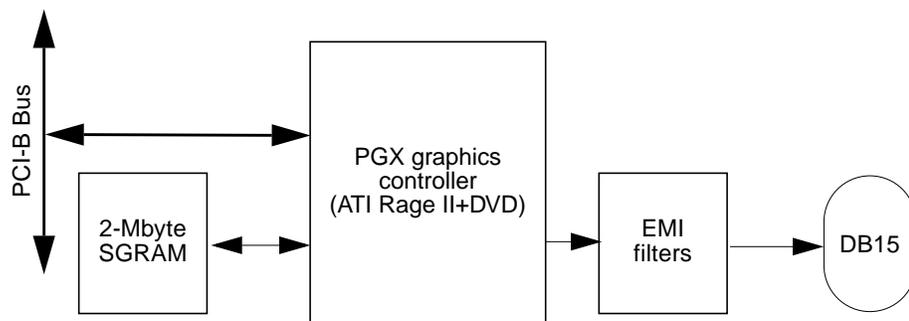
FIGURE C-7 PCI-Based Graphics Functional Block Diagram (PGX)
